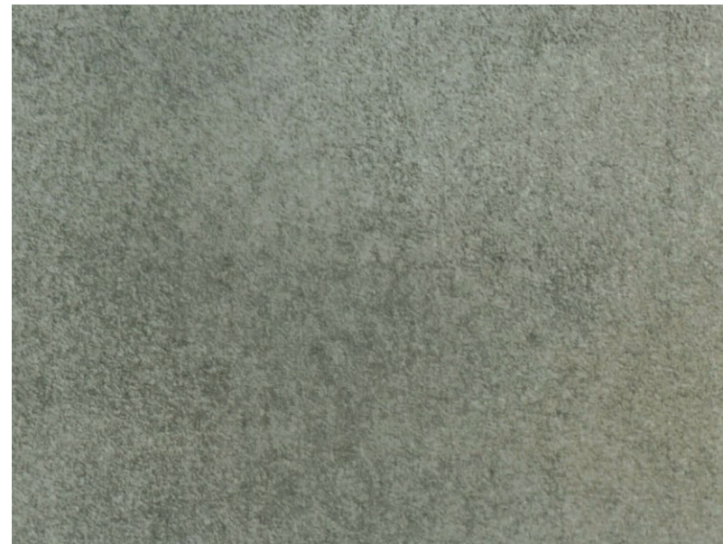
Preparation grades. Blast cleaning C Sa 2½
