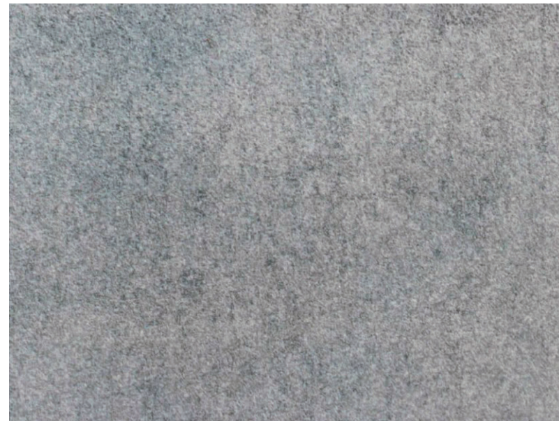
Preparation grades. Blast cleaning A Sa 2½
