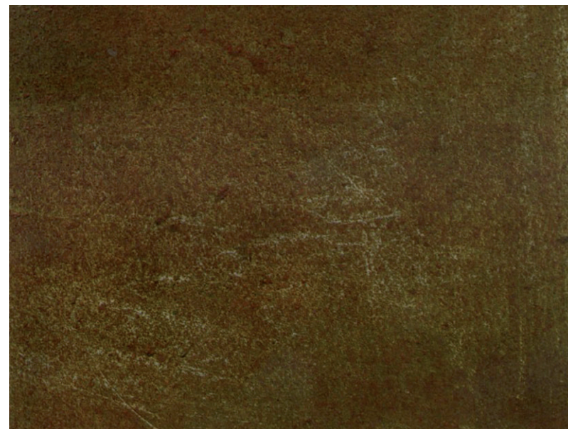
Preparation Grades. Scraping and wire-brushing C St 3
