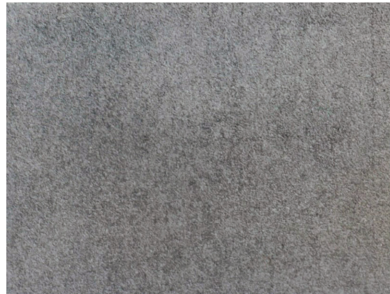
Preparation grades. Blast cleaning B Sa 2½
