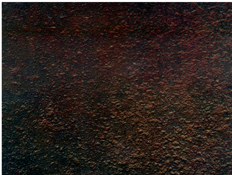
Preparation Grades. Scraping and wire-brushing D St 3
