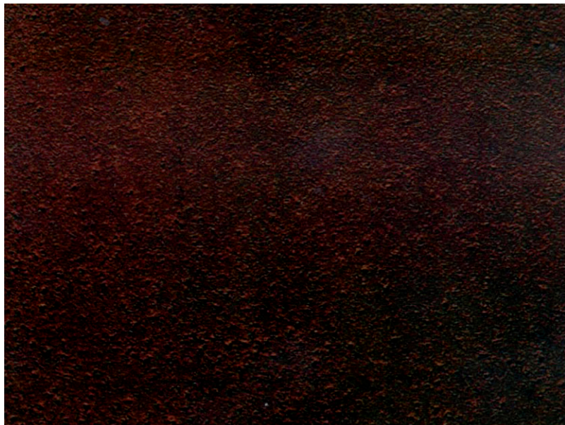
Preparation grades. Blast cleaning C Sa 1
