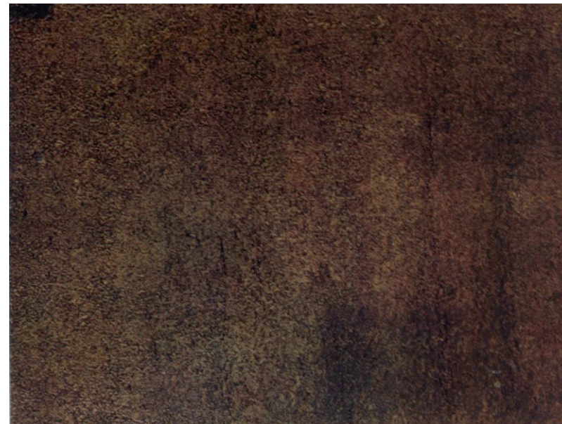
Preparation Grades. Scraping and wire-brushing C St 2
