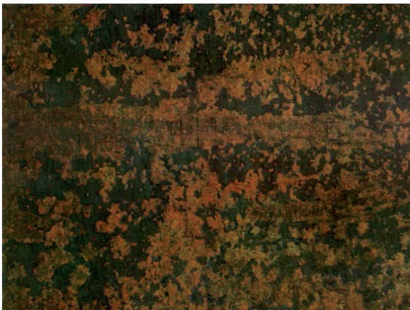
Preparation Grades. Scraping and wire-brushing B St 3
