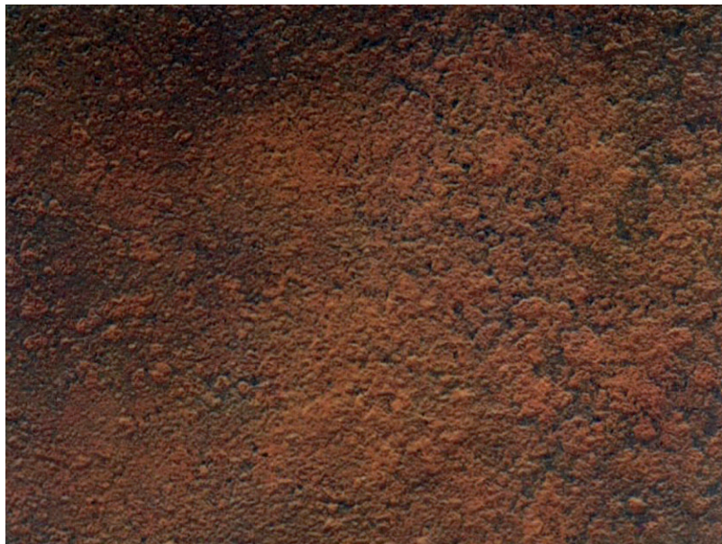
Preparation Grades. Scraping and wire-brushing D St 2
