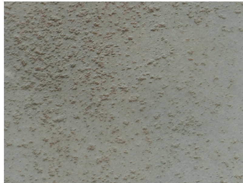
Preparation grades. Blast cleaning D Sa 2½
